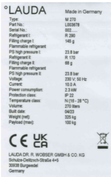
Fig. 16: Example of rating label
