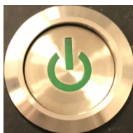
Fig. 12: Main battery switch pressed
