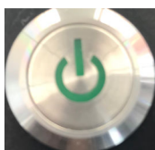
Fig. 32: Main battery switch
